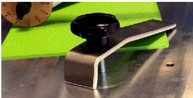
Universal Sample Clamp for flat and curved samples with various height
