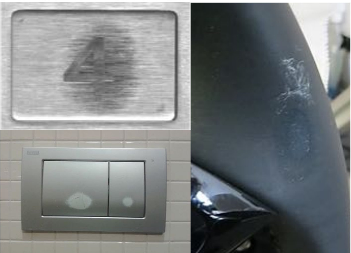
Examples of ABREX® - abrasion on button of ATM machine; steering wheel; toilet panel
